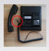
3. Plug the longer end of the cord into the furthest right port of the phone. It is marked with the handset symbol (in the yellow circles).
